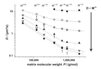
**Figure 3.** Dependence of the diffusion coefficient of several polymer tracers on matrix molecular weight in semidilute solution,  $c = 100 \text{ g L}^{-1}$ . Tracer molecular weights: ■: 50 000 g mol<sup>-1</sup>,  $\bigcirc$ : 123 000 g mol<sup>-1</sup>,  $\bigcirc$ : 200 000 g mol<sup>-1</sup>,  $\bigcirc$ : 390 000 g mol<sup>-1</sup>,  $\bigcirc$ : 650 000 g mol<sup>-1</sup>,  $\bigcirc$ : 900 000 g mol<sup>-1</sup>. Arrows indicate the situation when M = P.
