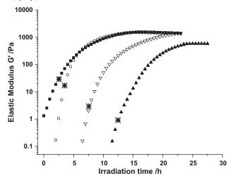
Figure 4. Elastic modulus G' (1 Hz) as a function of irradiation time (progress of photocross-linking) for four different matrices with similar degree of functionalization,  $C = 100 \text{ g L}^{-1}$ . Matrix molecular weight P:  $\triangle$ : 123 000 g mol $^{-1}$ ,  $\bigcirc$ : 200 000 g mol $^{-1}$ ,  $\bigcirc$ : 390 000 g mol $^{-1}$ ,  $\bigcirc$ : 900 000 g mol $^{-1}$ . Asterisks indicate G' = G'' (≈ gelation threshold).
