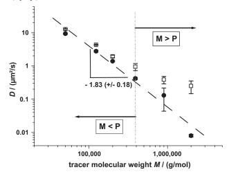
**Figure 6.** Dependence of the diffusion coefficient on the molecular weight of the polymer tracer in  $P = 390\,000\,\mathrm{g}\,\mathrm{mol}^{-1}$  P(s-co-ams);  $c = 100\,\mathrm{g}\,\mathrm{L}^{-1}$ ;  $\square$ : sol state (before photocross-linking),  $\bullet$ : gel state (after photocross-linking).
